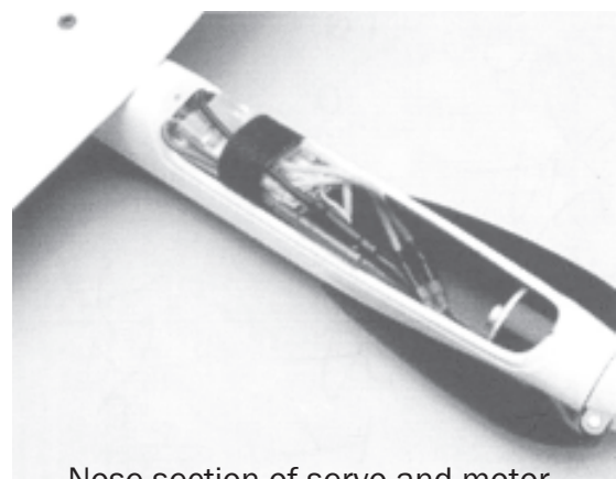
Nose section of servo and motor arrangement of electric version
